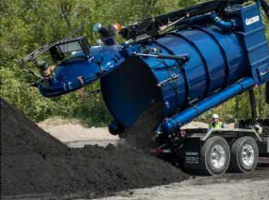
The new, rounded transition from debris body to cyclone allows the future addition of valving to isolate the tank for adding pressure offload systems. The new, full-opening door option further enhances the offload capabilities.
